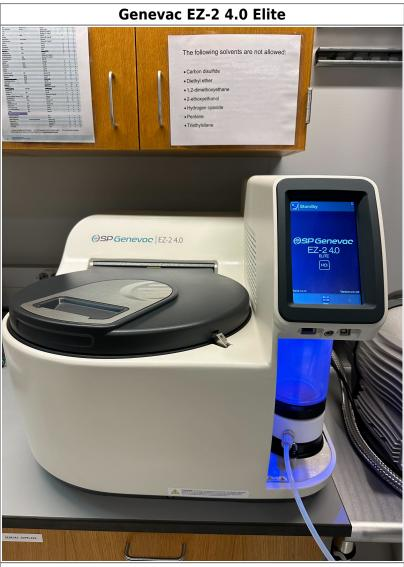
**Tool Type:** Parallel Evaporation System
