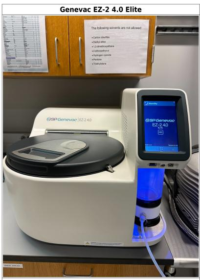
**Tool Type:** Parallel Evaporation System
