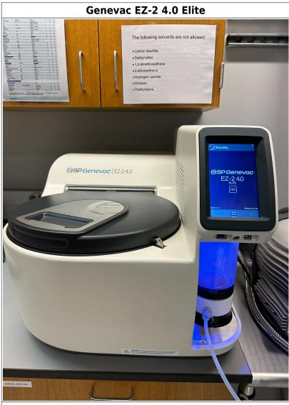
**Tool Type:** Parallel Evaporation System
