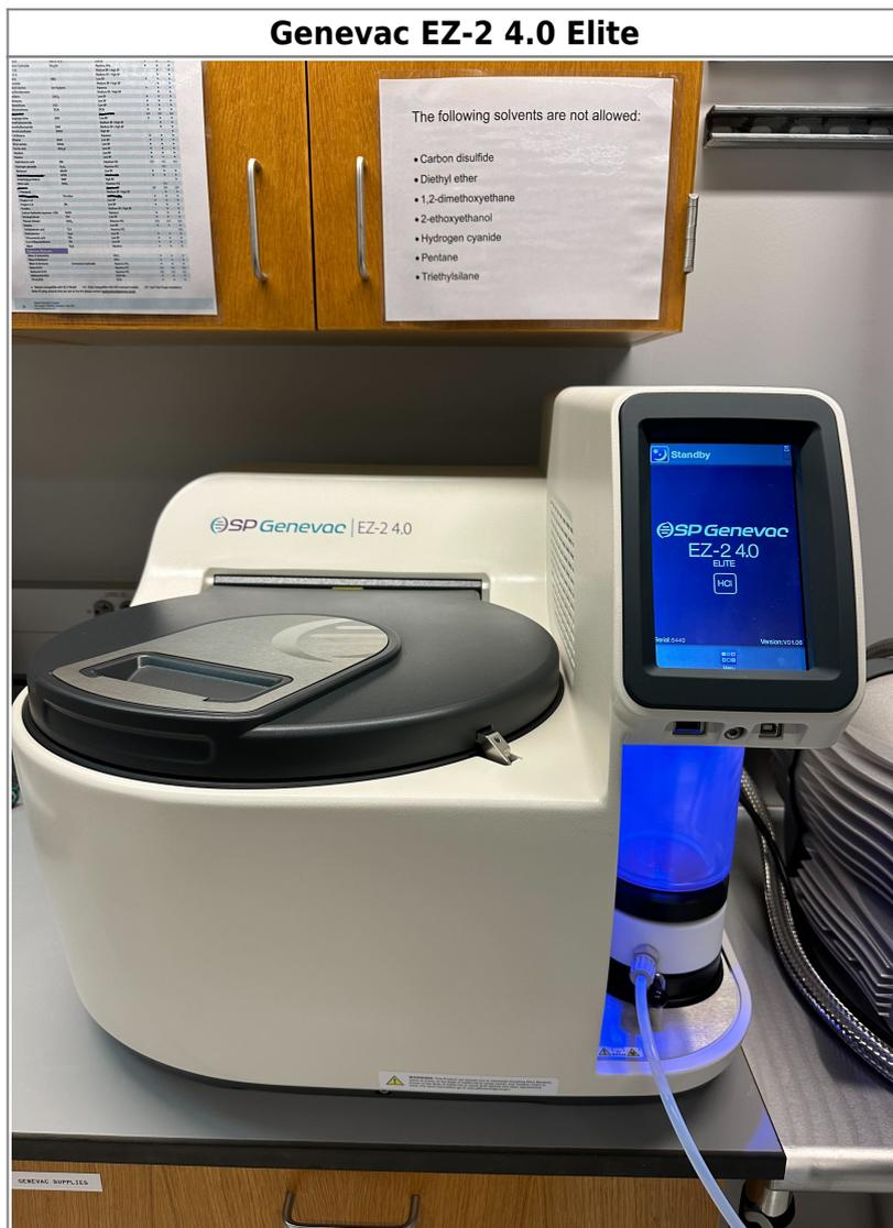
**Tool Type:** Parallel Evaporation System
