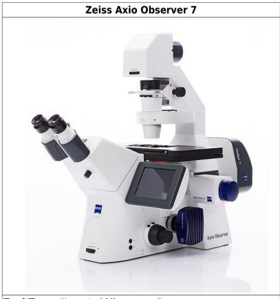
**Tool Type:** "Inverted Microscope"
