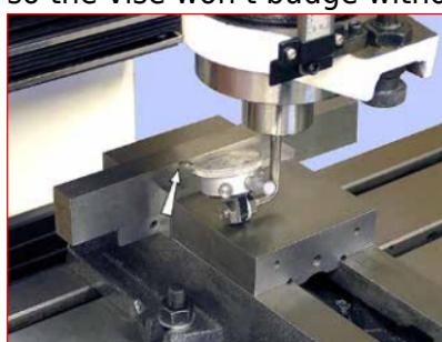
2. Adjust the Y-axis to pre-load the indicator to mid range at the tightly-clamped side of the vise, then lock the Y-axis. Do not allow the spindle to rotate during this procedure.
