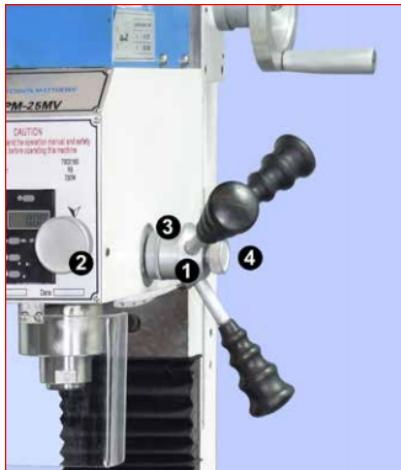
1. For drilling operations, loosen knob (4), allowing the lever hub to rotate independently of sleeve (3).
