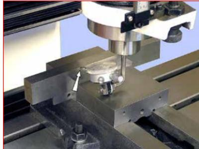
2. Adjust the Y-axis to pre-load the indicator to mid range at the tightly-clamped side of the vise, then lock the Y-axis. Do not allow the spindle to rotate during this procedure.
