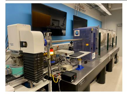
About the SAXS/WAXS Diffractometer
