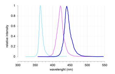
Typical spectral profile for each of the LED well plates available 365 nm, 420 nm, and 445 nm.
