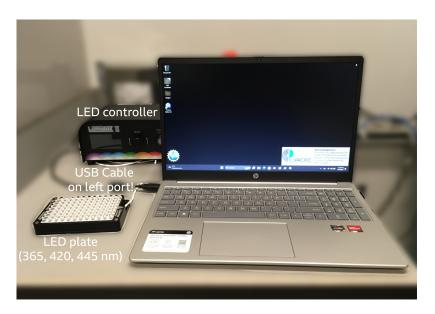
**NOTE** USB cable to controller needs to be connected on left port of computer for it to work properly with the computer.
