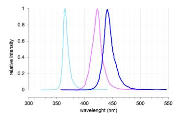
Typical spectral profile for each of the LED well plates available 365 nm, 420 nm, and 445 nm.
