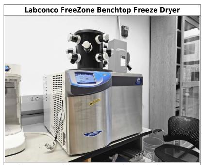
**Tool Type:** Material Processing, Drying, Annealing
