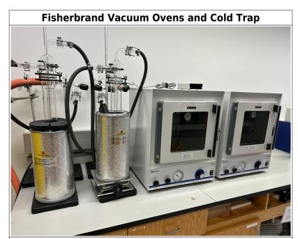
**Tool Type:** Material Processing, Drying, Annealing
