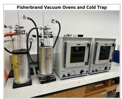
Tool Type: Material Processing, Drying, Annealing
