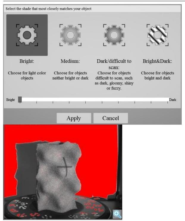
• Once a texture mode is selected, the brightness slider will appear. Use the camera screen in the upper right as a reference for adjusting the brightness level. Move the slider so that the crosshair is clearly illuminated on the object in the view window, but not so brightly illuminated that red areas show up on the object to be scanned. An example image of the right exposure over the part is shown.
