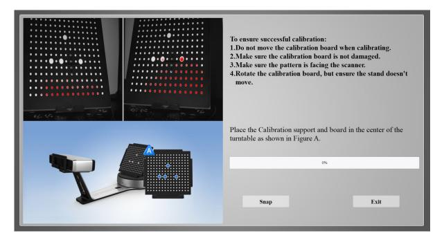
• This menu will appear. Remove the calibration board from the black protective drawstring bag and snap together the calibration board stand. Place the stand in the center of the turntable facing the scanner, and mount the calibration board in Orientation A (specified by the software). When properly oriented, click Snap \_\_\_\_\_ to proceed. The turntable will incrementally rotate and
