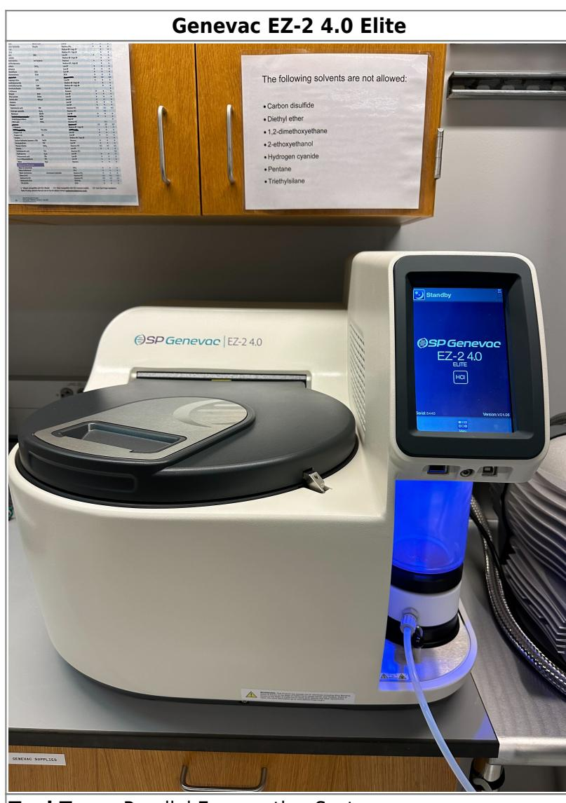
**Tool Type:** Parallel Evaporation System
