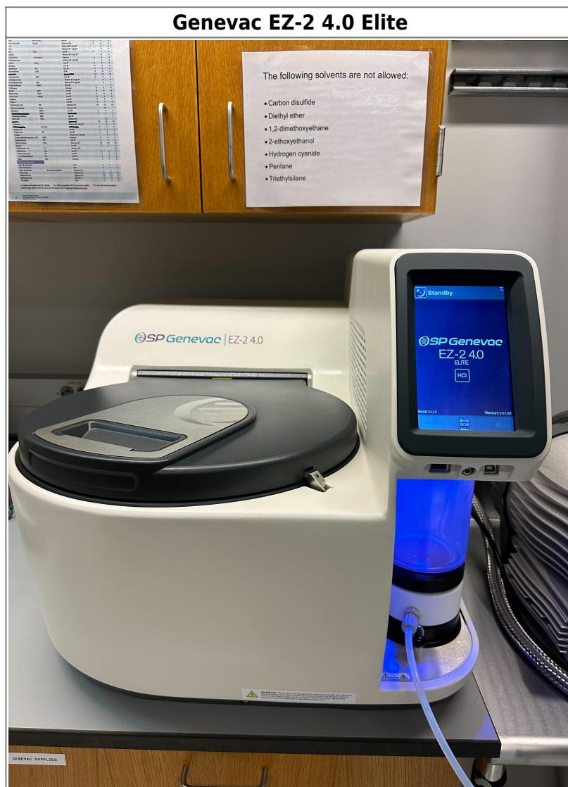
**Tool Type:** Parallel Evaporation System
