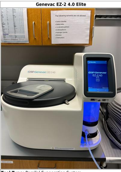
Tool Type: Parallel Evaporation System
