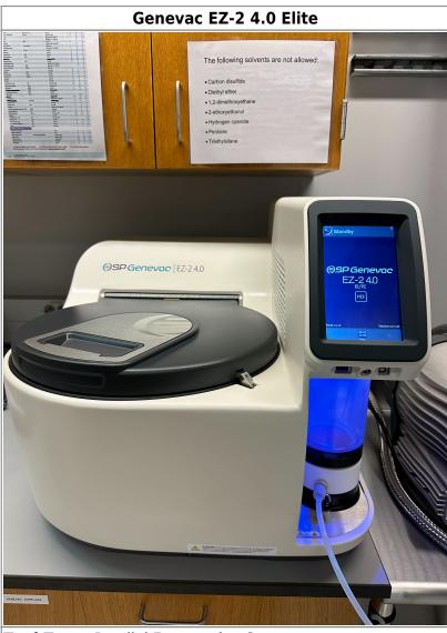
Tool Type: Parallel Evaporation System
