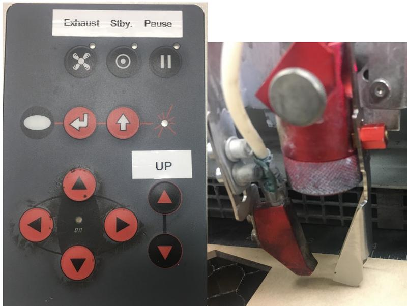
4. Using the arrow pad, **position the head of the laser where you want the top left corner of your print to begin on the material.**
