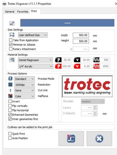
10. Open Job Control and connect to the printer by clicking the USB symbol.
