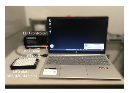
**NOTE** USB cable to controller needs to be connected on left port of computer for it to work properly with the computer.
