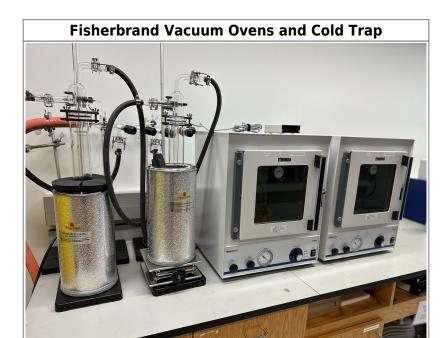
**Tool Type:** Material Processing, Drying, Annealing
