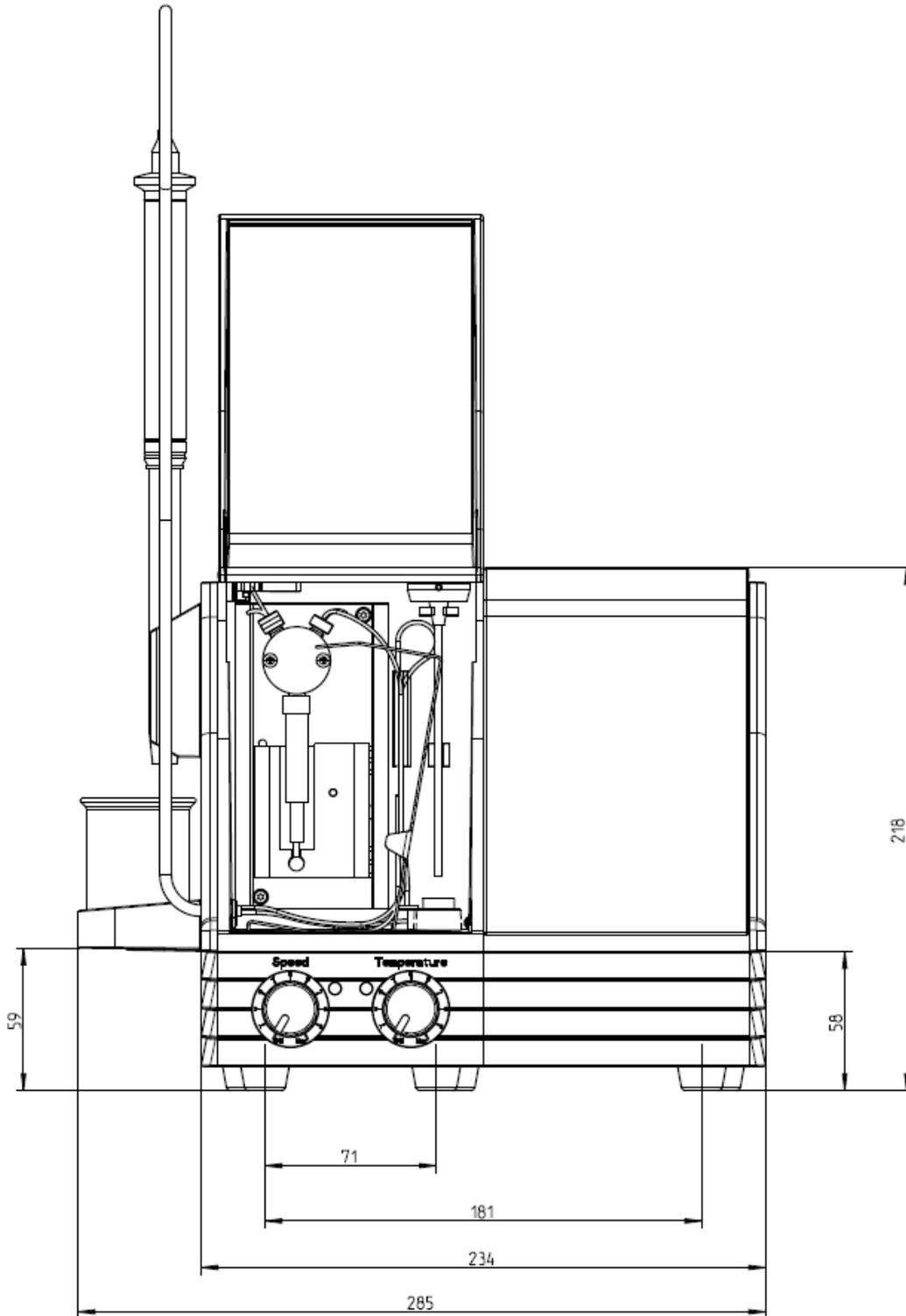
Two Syringe Injector with Heater Stirrer - Side View
