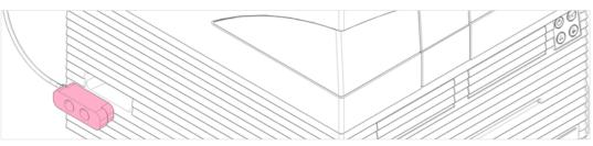
Figure 105: Condensation prevention stoppers (both sides of the instrument)
