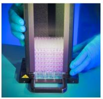
4. Lift up the plate magazine. The stack of microplates has been added to the plate magazine. The platform plate remains on the lab bench.
