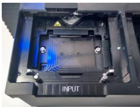
3. Place the microplate on the center of plate transport. Ensure that the **A1** label on the microplate is in the upper left hand corner. Always place the microplate on the plate transport – never directly onto the lifting table of the stacker.
