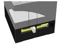
4. Move the plate carrier out carefully by hand until it lightly presses against the inserted white piece of foam from behind and cannot be moved out further.
