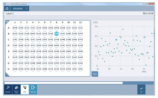
Figure 21: Monitoring a single-label endpoint measurement
