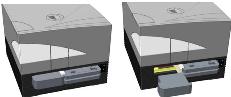
4. Move the plate carrier out manually by pulling on the pieces of foam in the right plate carrier compartment (see picture below).
