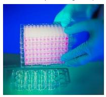
3. Slide the plate magazine over the stack of microplates all the way down until the plate magazine makes contact with the surface of the lab bench.
