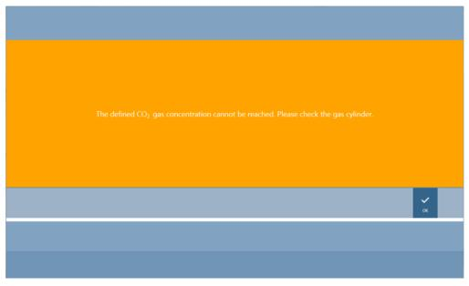
Figure 109: Stopping the gas alarm
