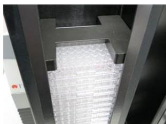
2. Place a stabilizer weight at the bottom of the output magazine.
