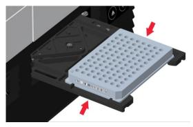
Apply the barcode on the left or right side of the microplate.
