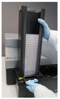
3. Load the empty plate magazine at the position labelled OUTPUT.
