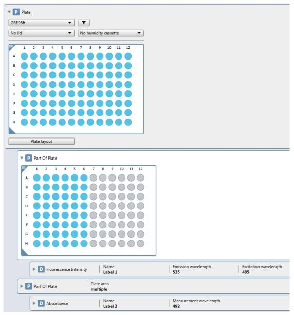
Figure 7: (Plate: A1-H12; Part of Plate: A1-H6; FI; Part of Plate: A7-H12; ABS)
