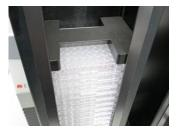
2. Place a stabilizer weight at the bottom of the output magazine.
