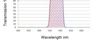
Figure 30: The combination of a 505 nm long pass filter with a 575 nm short pass filter yields a spectral measurement window for the luminescence emission from 505 to 575 nm.
