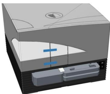
3. Remove the piece of foam from the left plate carrier compartment (see picture below).
