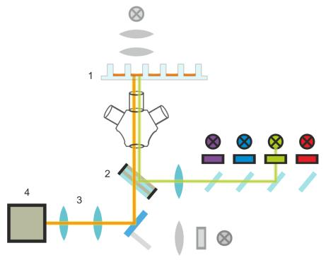
Figure 72: Schematic diagram of the fluorescence illumination system
