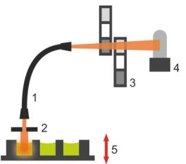
Figure 31: Optical system in luminescence enhanced module:[1] luminescence fiber, [2] aperture wheel,[3] two filter wheels, [4] detection unit, [5] z-drive of plate transport
