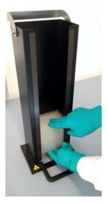
Carefully slide one hand underneath the microplate at the bottom of the plate magazine, and stabilize the group of microplates you want to unload, with the other hand.
