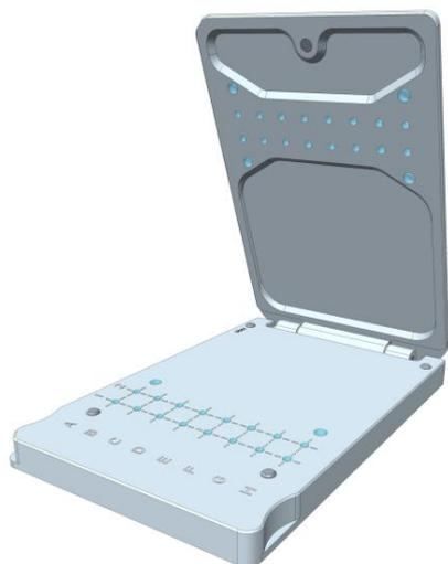
Figure 45: NanoQuant Plate
