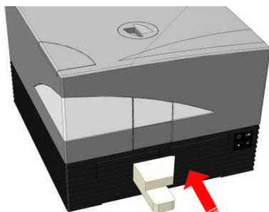
3. With the foam piece inserted, turn it 90° clockwise, so that the pointed end sticks down into the space between the two compartment openings. This piece of foam holds the compartment doors open.
