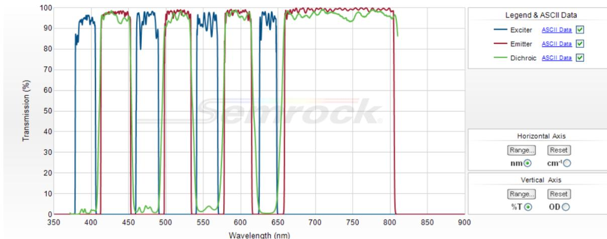
Figure 73 Transmission profile of the full-multiband filter set, built-in T-image (obtained from the official Semrock website: [www.semrock.com](http://www.semrock.com)).
