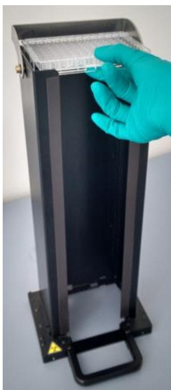
1. Manually insert the microplate into the top of the plate magazine and carefully lower it towards the bottom of the plate magazine.
