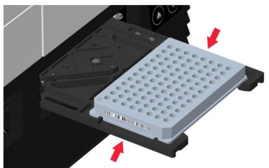
Apply the barcode on the left or right side of the microplate.
