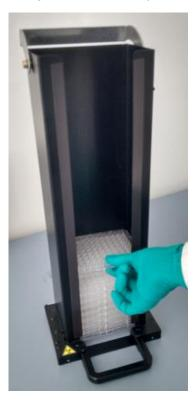
2. Carefully grip the microplate at the top of the stack of plates in the plate magazine.
