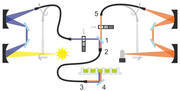
Figure 49: Fluorescence bottom module – monochromator option highlighted
