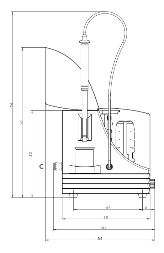
Two Syringe Injector with Heater Stirrer - Side View
