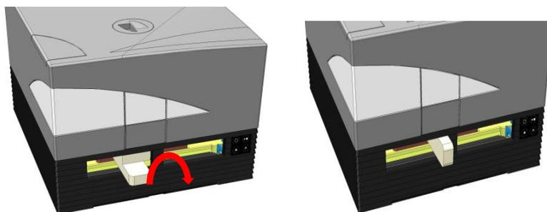
4. Move the plate carrier out carefully by hand until it lightly presses against the inserted white piece of foam from behind and cannot be moved out further.
