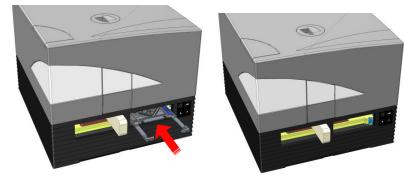
7. Rotate the remaining piece of foam 90° counter-clockwise and pull it out of the instrument (see picture below).
