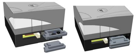
6. Move the plate carrier into the right compartment manually as far as it can go by pushing on the pieces of foam on the plate carrier.
