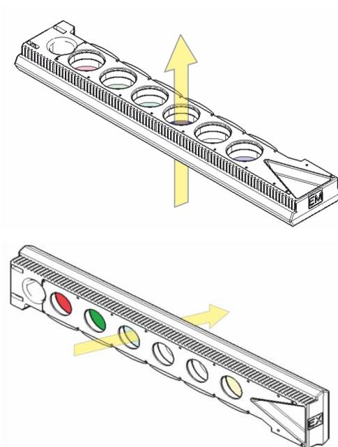
Figure 51: Direction of light through the filter slides
