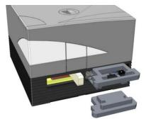
6. Move the plate carrier in carefully by hand. It must be pushed in far enough so that the plate carrier compartment door can close (see picture below).
