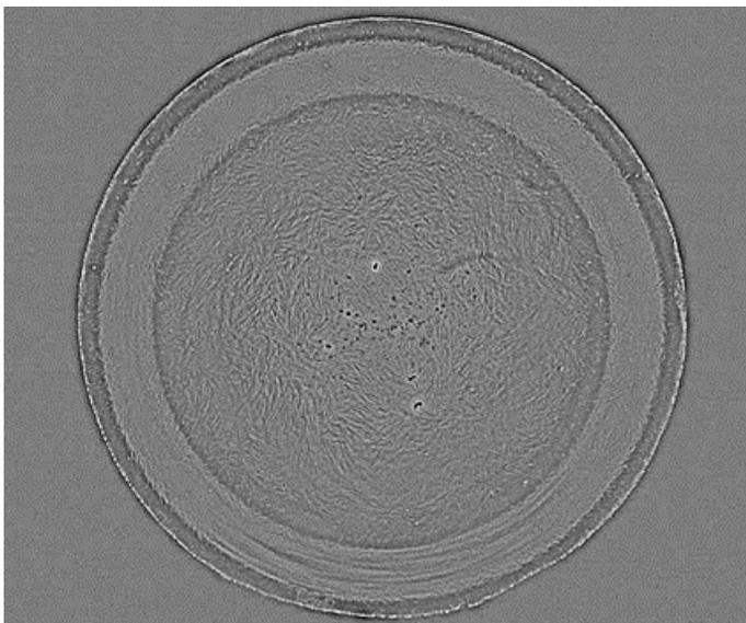
Figure 76 Processed bright field image of a well (96 well microplate) filled with 100 µl of medium.
