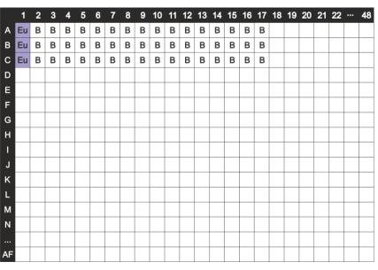
Eu: 10 μl 1 nM Europium (Monochromator) / 0.1 nM Europium (Filter) B: 10 μl Blank (Enhancement Solution)
