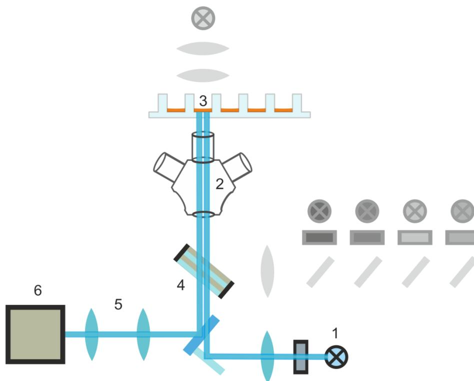
Figure 71: Schematic diagram of the auto-focusing system
