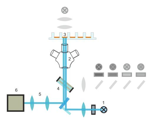
Figure 71: Schematic diagram of the auto-focusing system
