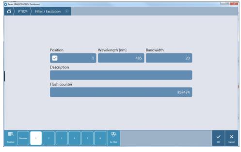
Figure 55: Defining a filter for position 1
