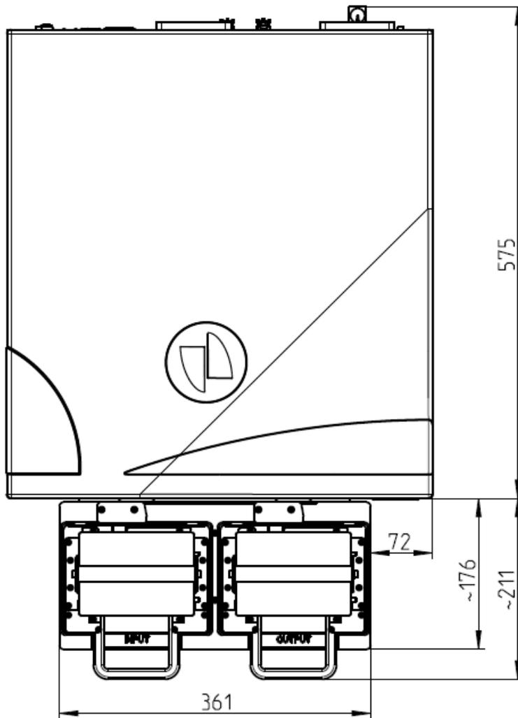
**SPARK with Spark-Stack – Rear View**
