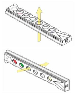
Figure 51: Direction of light through the filter slides
