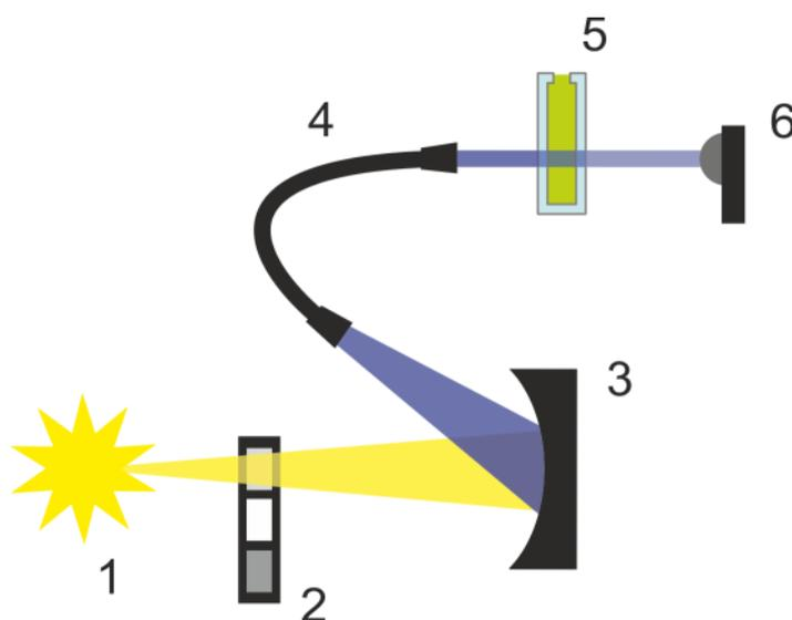
Figure 39: Optical system absorbance cuvette module
