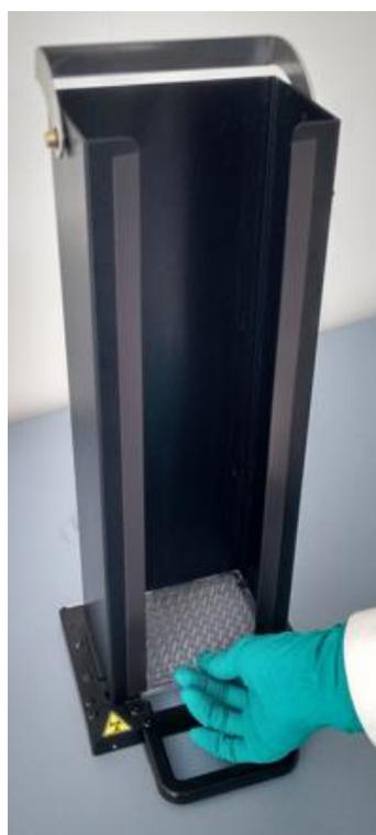
2. Gently release the microplate at the bottom of the plate magazine.
