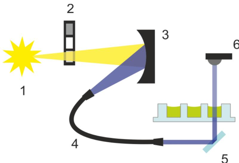
Figure 38: Optical system in absorbance module
