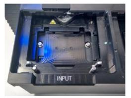
3. Place the microplate on the center of plate transport. Ensure that the **A1** label on the microplate is in the upper left hand corner. Always place the microplate on the plate transport – never directly onto the lifting table of the stacker.
