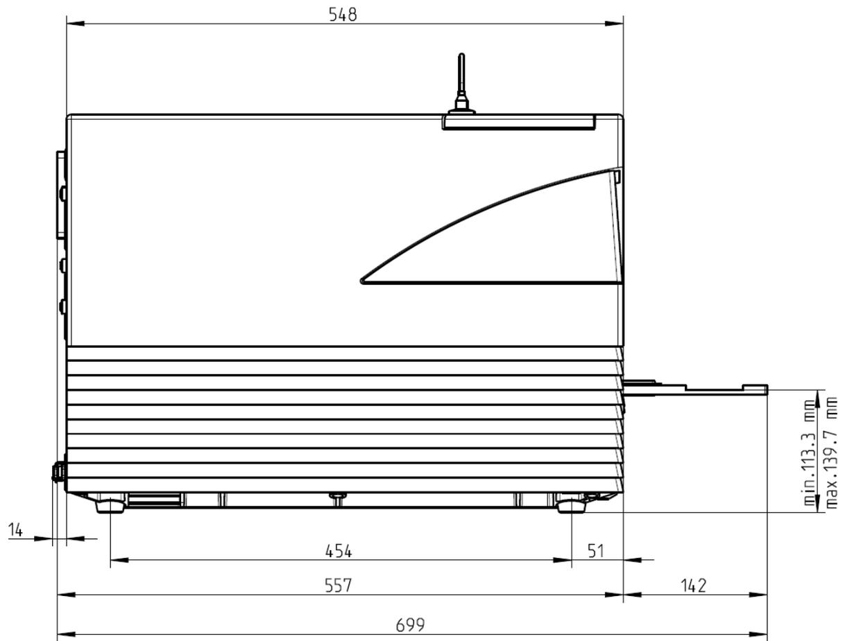
**Two Syringe Injector with Heater Stirrer - Front View**
