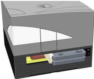
7. Insert the piece of foam into the left plate carrier compartment (see picture below).
