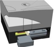
4. Move the plate carrier out manually by pulling on the pieces of foam in the right plate carrier compartment (see picture below).
