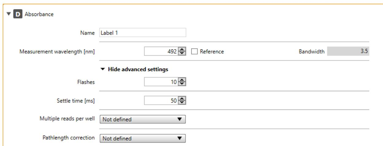
Figure 43: Absorbance strip for absorbance module
