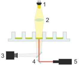
Figure 64: Cell counting optics LED [1], lens system [2], camera [3], mirror [4], laser diode [5]
