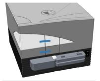
3. Remove the piece of foam from the left plate carrier compartment (see picture below).
