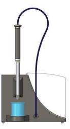
Figure 89: Injector carrier in service position
