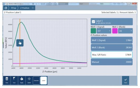
Figure 62: Z-Position window – display of Z-position curves
