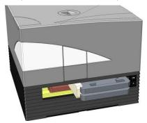
7. Insert the piece of foam into the left plate carrier compartment (see picture below).
