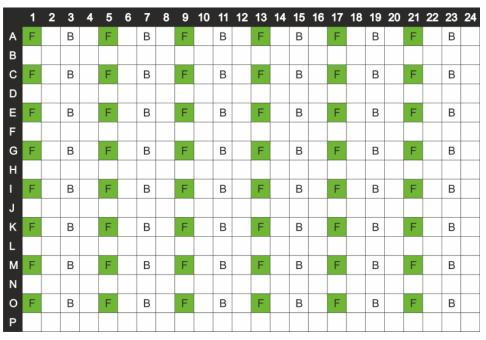
F: 100 µl 1 nM Fluorescein B: 100 µl Blank (10 mM NaOH)
