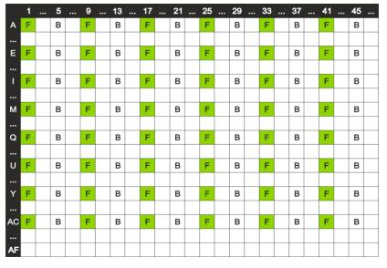
F: 10 µl 1 nM Fluorescein B: 10 µl Blank (10 mM NaOH)
