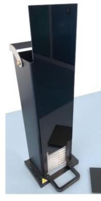
1. Place the front cover onto the magnetic strips of the plate magazine.
