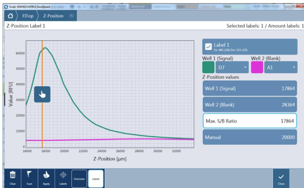
Figure 62: Z-Position window – display of Z-position curves
