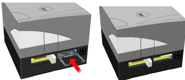
7. Rotate the remaining piece of foam 90° counter-clockwise and pull it out of the instrument (see picture below).
