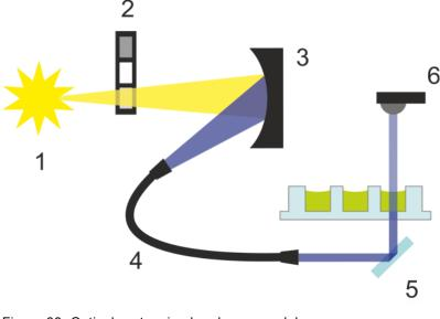
At the focal point the spot diameter of the absorbance light beam is about 1 mm.
