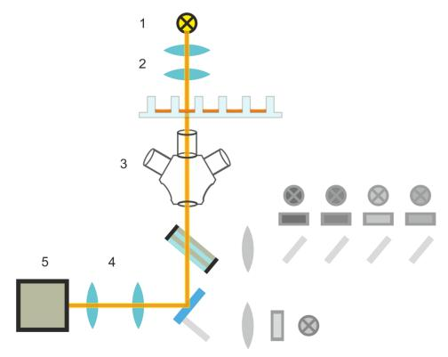
Figure 70: Schematic diagram of the bright field illumination system
