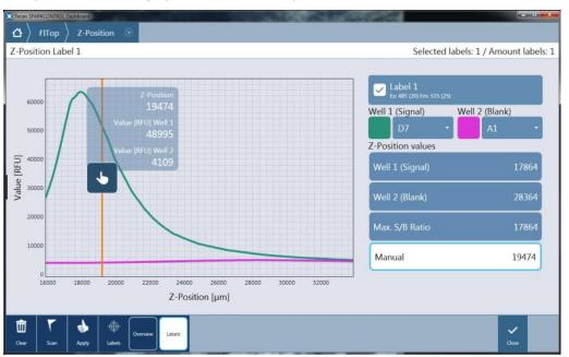
Figure 63: Z-Position window – changing Z-position value manually
