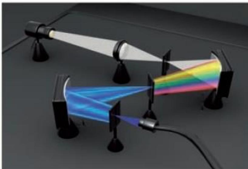
Figure 46: Double monochromator concept
