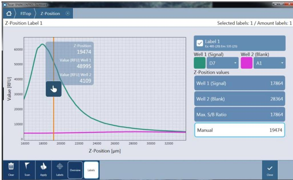
Figure 63: Z-Position window – changing Z-position value manually
