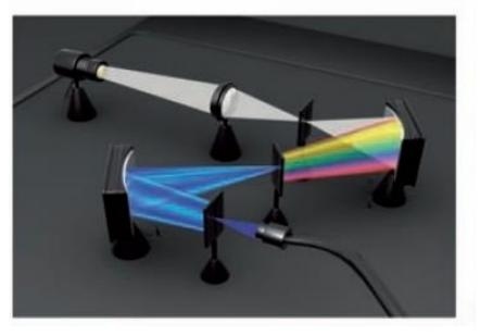
Figure 46: Double monochromator concept
