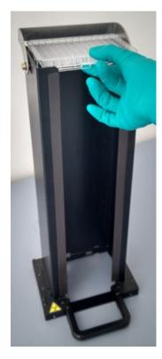
Manually insert the microplate into the top of the plate magazine and carefully lower it towards the bottom of the plate magazine.
