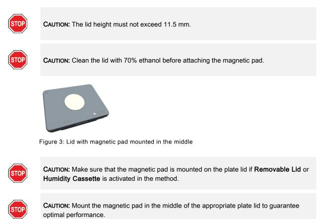
The lid lifter option is used to temporarily remove the lid of the microplate to execute, e.g. injection steps or measurement steps within the workflow of a long term experiment thus avoiding sample evaporation.
