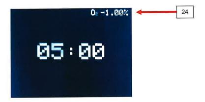
After the start button is pressed, the nitrogen valve opens and the chamber is purged. While the  $O_2$  level is above the pre-set value (default is 4%), the start button flashes and the rotation stage and LEDs are disabled.
