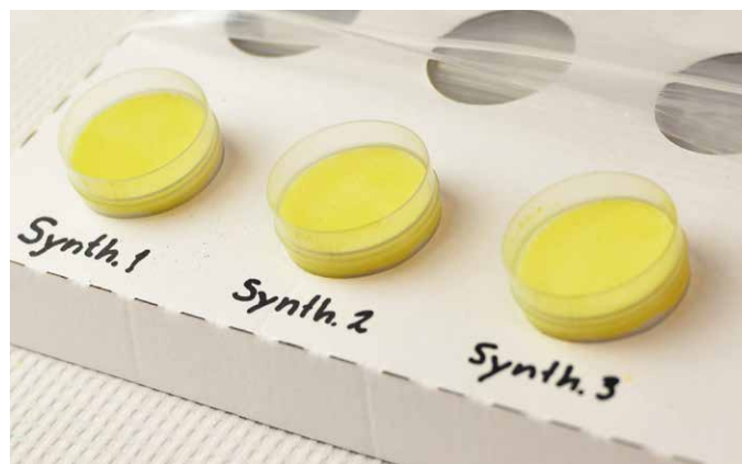
Figure 6. If several Samplet® cartridges are to be prepared at the same time, labels or descriptions can be written on the cardboard shipping material by each Samplet®.
