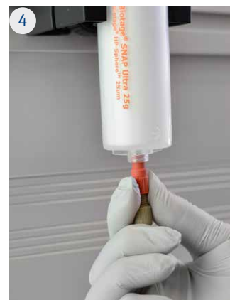
Twist the Luer fitting on securely to the bottom of the cartridge.
