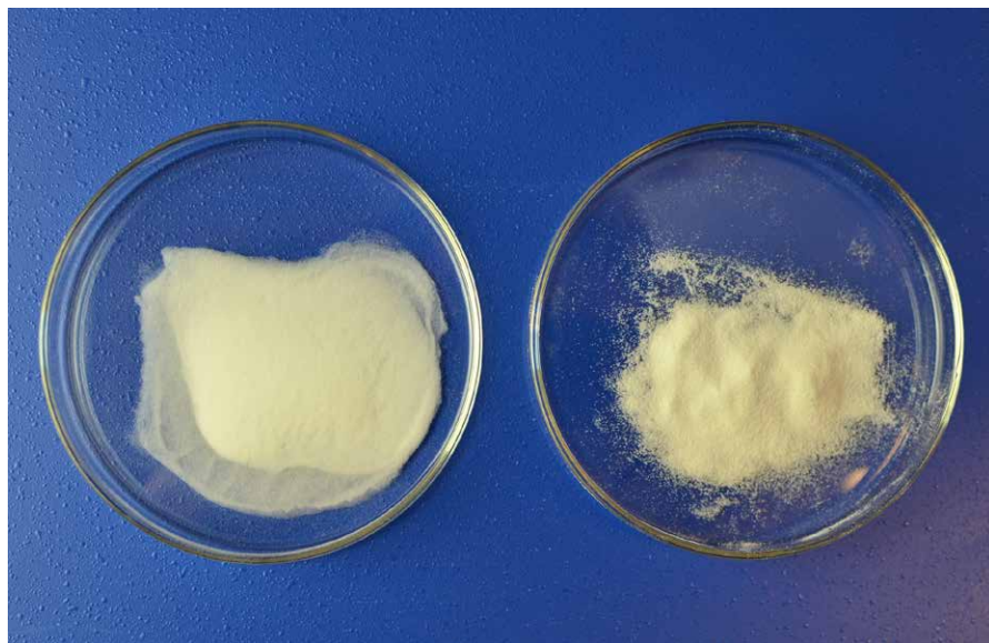
Figure 1. Left: Pre-adsorption on silica gel (3 g, part number K0-1107-05000). Right: Pre-adsorption on Biotage HM-N diatomaceous earth (3 g, part number 9800-1000).
