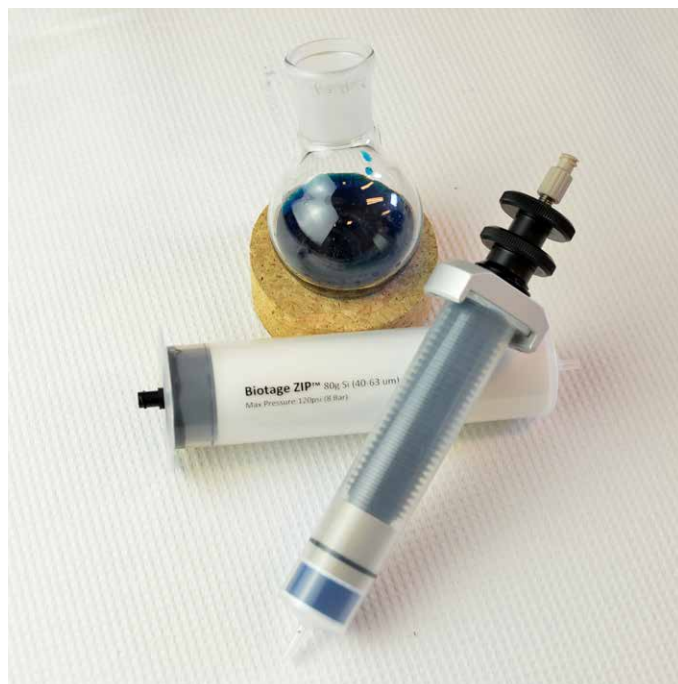
Figure 5. After evaporation of the solvent, dried adsorbent is poured into empty Dry Load Vessels which can be connected to any Biotage cartridge.
