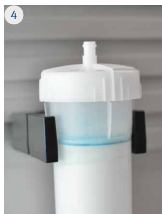
Cap fully tightened showing 1 mm gap between the cap and mounting fin.
