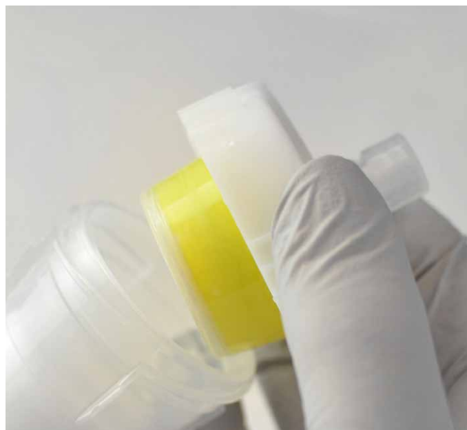
Figure 4. Samplets are placed inside of Biotage® SNAP cartridges which maximizes the amount of media available for purification and eliminates and precipitation risk.
