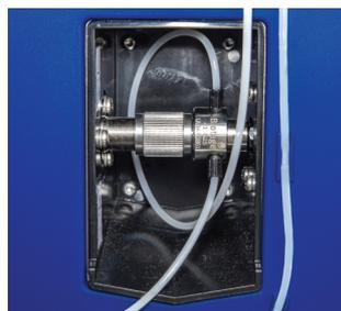
Figure 58. Drainage of leakage from the flow cell of the internal detector.
