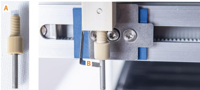
Figure 63. Assemble the needle, ferrule (A), and nut, and assemble it on the collection arm. Ensure that the needle is touching the needle guide (B).
