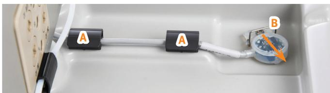
**Figure 59.** Instrument tray with a solvent detector. A = tube clips holding the detector cable and B = the solvent detector hatch open.
