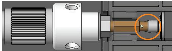
**Figure 55.** Cross section of the flow cell properly inserted into the UV detector.
