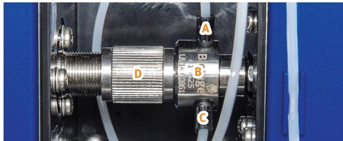
**Figure 54.** The flow cell of the internal detector. A = flow cell outlet tube, B = flow cell, C = flow cell inlet tube, and D = retaining nut.
