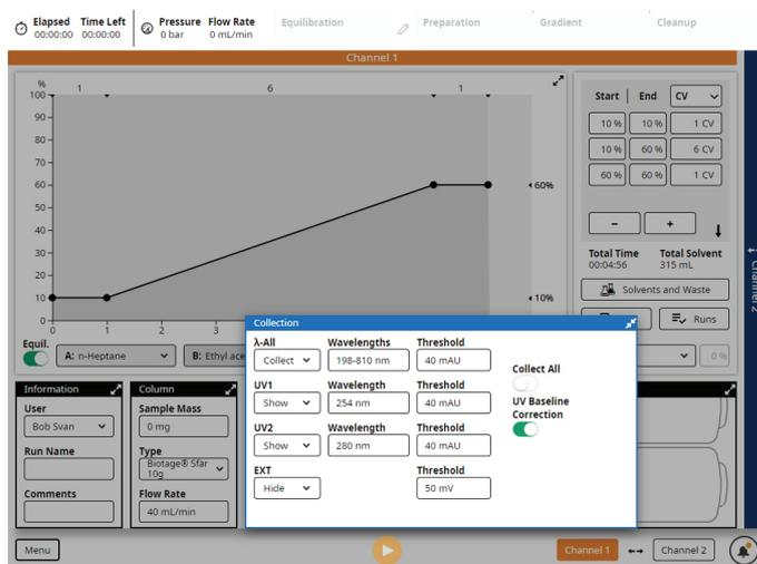
Figure 6. The Collection panel expanded on a system with a Spektra software license and an external detector connected.
