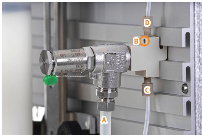
**Figure 11.** The safety valve. A: Drain tube. B: Screw for fastening the valve to the system. C: Tube from the C1 or C2 port on the right side of the system. D: Tube going to the top of the column.
