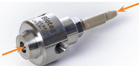
**Figure 53.** The fiber optics on the flow cell. Do not touch.
