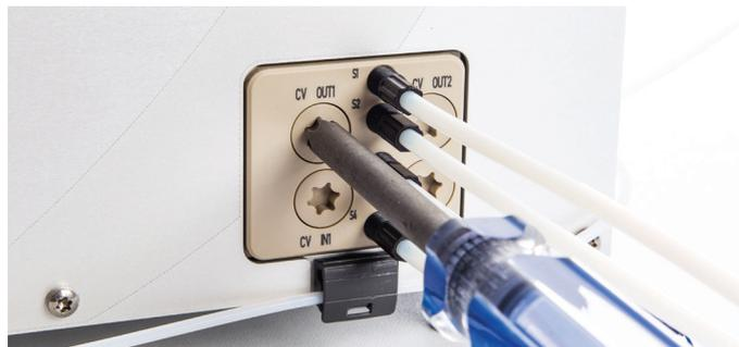
Figure 64. Removing the check valve cap from one of the CV OUT valves.
