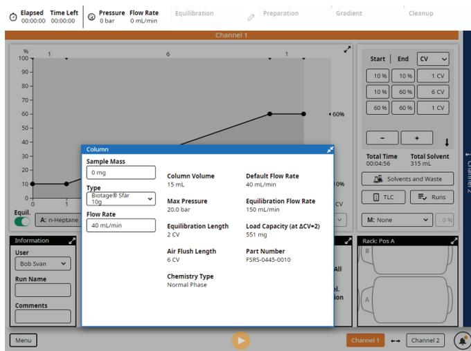
Figure 24. The Column panel expanded.
