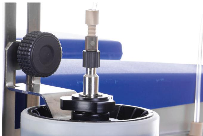
**Figure 13.** The top screw is used for adjusting the column holder to the length of the used column.
