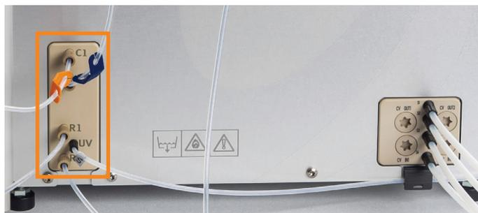
Figure 15. The C1, C2, R1, and R2 ports on the right side of the system.
