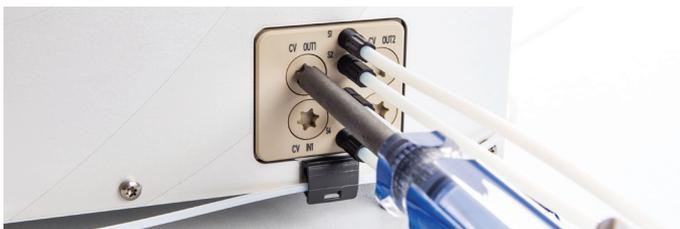
Figure 56. Removing the check valve cap from one of the CV OUT valves.
