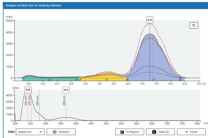
**Figure 39.** The Analysis view showing the chromatogram and the absorbance spectrum. Requires a Spektra software license.
