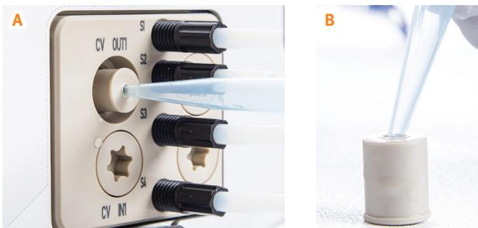
Figure 57. Release stuck check valves.
