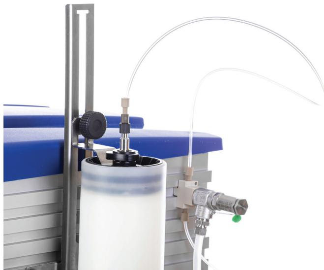
**Figure 8.** The safety valve connected to a SNAP XL column mounted on the system.
