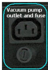
6. **Important!** When installing BioTek's vacuum pump, connect the pump's AC power cable to the vacuum pump **Accessory Outlet** on the back of the instrument. (Use the accessory outlet adapter provided, if applicable.)
