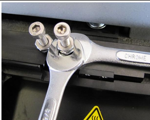
One wrench per nut to tighten top one
