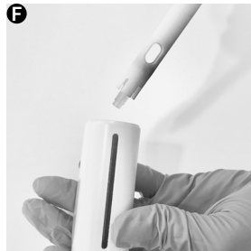
Figure 7: Removing the Luer lock adapter. (A, D) Insert the removal tool into the EMD printhead. (B, E) Fit the Luer lock and twist counterclockwise until loose. (C, F) Pull out and remove the adapter.
