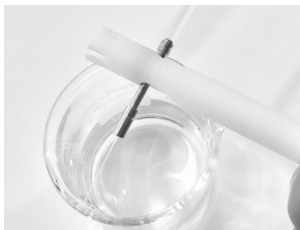
Figure 26: Flushing the microvalve.
