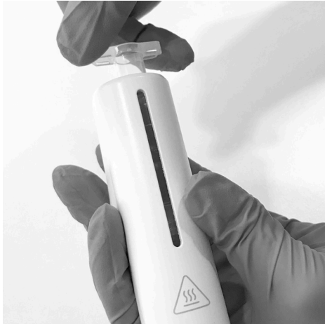
Figure 10: Inserting and tightening the cartridge into the EMD Printhead.
