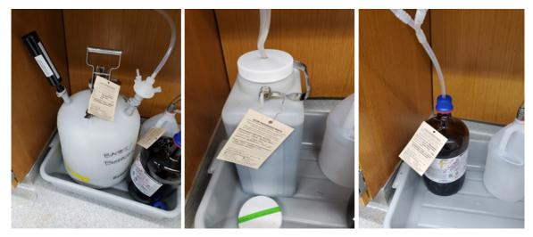
In the left photo, tubing is connected via a hose barb adapter for the container shown. The middle photo shows a reusable white 9 L container provided by EH&S that should only be used for HPLC eluent waste. The right photo shows how to connect a recycled 4 L solvent bottle as a waste reservoir. Spare caps with drilled holes for inserting the waste line are located in the secondary containment tub.
