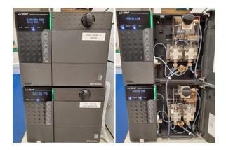
Watch for any bubbles in the lines and let these pass through the piston heads of the pumps for removal. Press the purge button again to stop purging. Remember to close the black valve finger-tight. Do not close too tightly or you may damage the pump.
