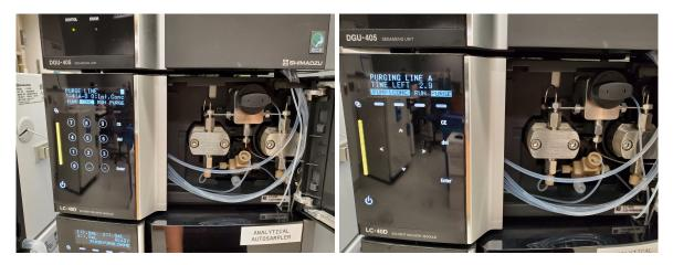
Repeat for each additional solvent line. Once the purging is complete, remember to close the black valve finger-tight. *Do not close too tightly or you may damage the pump.*
