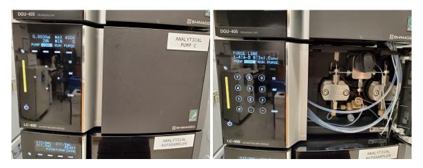
Press the purge button and type the number of the solvent line you would like to purge (e.g., 1 =Solvent A, 2 =Solvent B, 3 =Solvent C, 4 =Solvent D). Press Enter.
