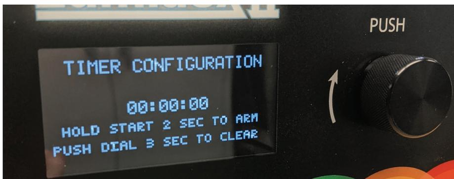
To enable the countdown timer, select the menu by pressing the center control knob (“PUSH”) once while on the home screen. Follow the on-screen directions to configure time. Press and hold *START/CANCEL* for 2 seconds to arm. **Ensure safety goggles and shields are in place.** Press *START/CANCEL* again to illuminate. Remaining time is displayed in the upper right of the screen.
