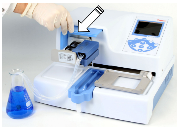
Figure 4–20. Pulling the rotor cover over the rotor
