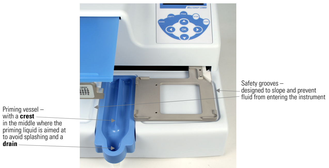
Figure 4–9. Priming vessel inserted into place
