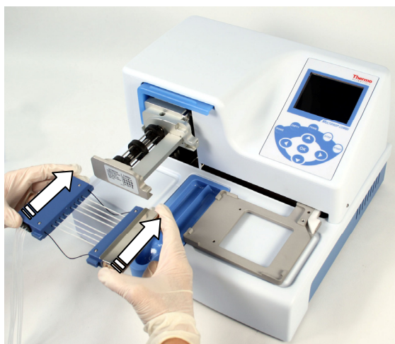
Figure 4–11. Inserting the dispensing cassette
