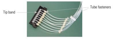
**Figure 5–29.** Inserting the tip manifold into the lower part of the dispensing cassette
