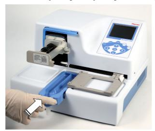
**Figure 3–8**. Inserting the priming vessel
