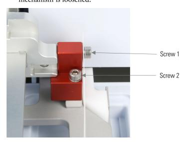
Figure 3-6. Transport lock fastened
