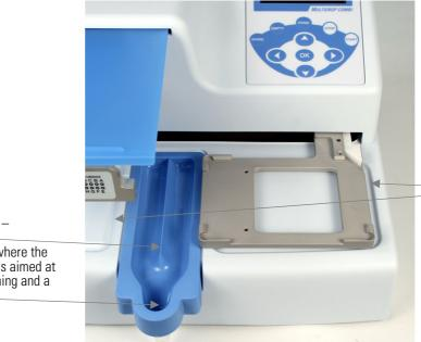
Safety grooves – designed to slope and prevent fluid from entering the instrument
