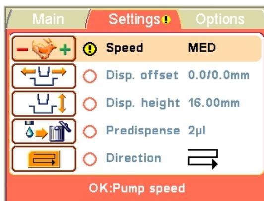
The changes made to the protocol settings only remain in the instrument memory if the protocol is saved with a name (see “Save and edit protocol” on page 51). If the protocol is not saved, the changes only remain effective until the plate type is changed or the instrument is switched off.
