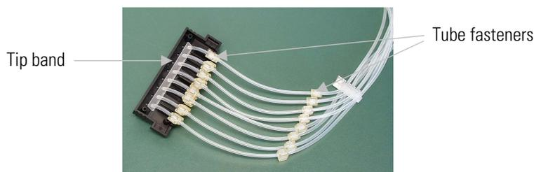
**Figure 5–29.** Inserting the tip manifold into the lower part of the dispensing cassette
