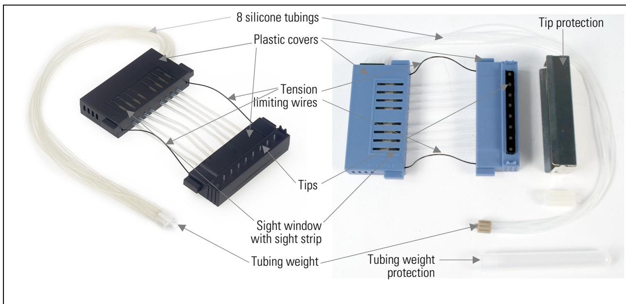
**Figure 4–10.** Parts of a dispensing cassette
