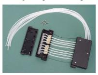
**Figure 5–24.** Removing the cover plate of the lower part of the dispensing cassette
