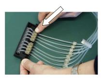
**Figure 5–30.** Pressing the tube fasteners into place
