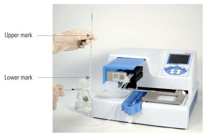
**Figure 6–52**. Adjusting the liquid level first to the lower mark and then to the upper mark
