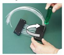
**Figure 5–42.** Fastening the cover retaining screws
