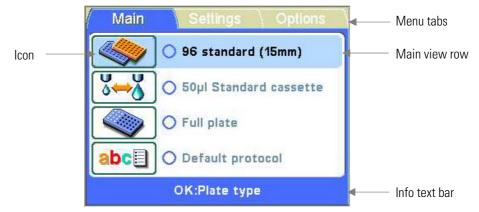
**Figure 4–22.** Main view on the display of the Multidrop Combi
