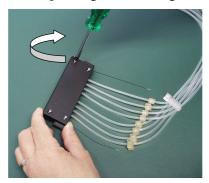
**Figure 5–33.** Replacing the lower part cover of the dispensing cassette
