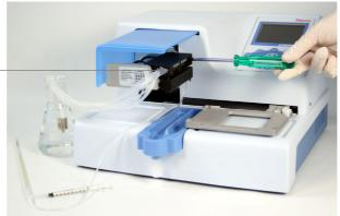
**Figure 6–53**. Screwing the calibration screws according to the calibration results
