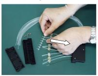
Figure 5–25. Removing the old tip band
