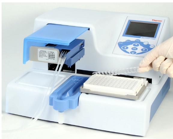
**Figure 6–49.** Removing the filled microstrip to be weighed
