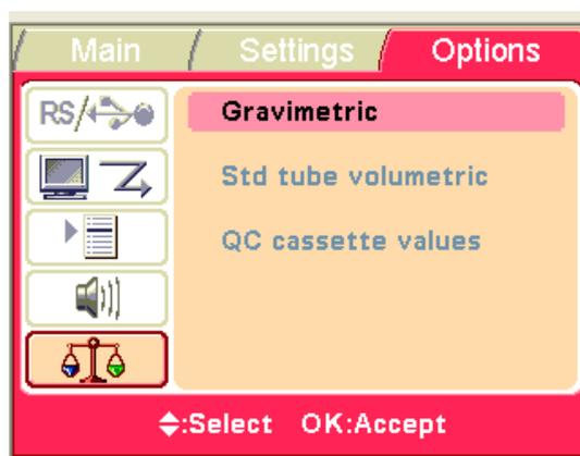
**Up** **Down** Use the **Up** and **Down** arrow keys to select the calibration mode. If a *SMART cassette* is used, the calibration data can be viewed.
