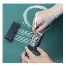
Figure 5–37. Pressing the tube fasteners into place
