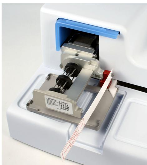
**Figure 3–5.** Transport lock and transport lock tag present
