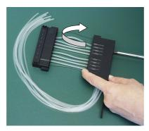
**Figure 5–46.** Precalibrating the dispensing cassette
