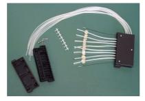
Figure 5-26. Tip band removed
