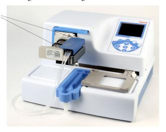
**Figure 4–14.** Lower and upper parts of the dispensing cassette inserted evenly into their slots
