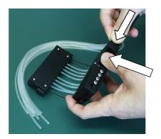
Figure 5–43. Inserting the cover on the calibration screws
