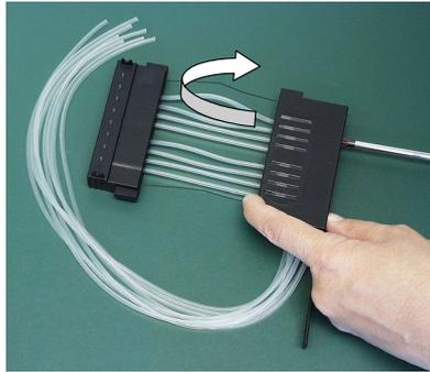
**Figure 5-46.** Precalibrating the dispensing cassette
