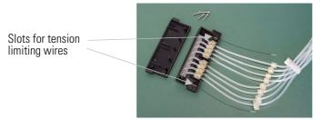
Figure 5–32. Tension limiting wires attached
