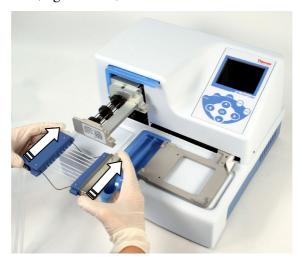
Figure 4–11. Inserting the dispensing cassette
