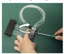
Figure 5–38. Fastening the calibration screws
