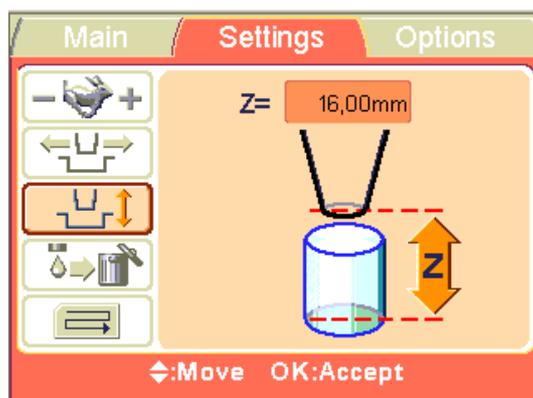
Use the **Up** and **Down** arrow keys to set the dispensing height. While you change the height, the pump body moves accordingly. The height is set in 0.05 mm increments in both the up and down directions. The minimum height value depends on the selected plate type (see Table 4–3). The default dispensing height is 1 mm above the selected plate.
