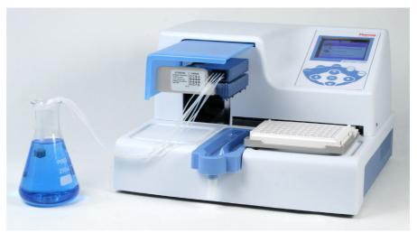
Figure 1–1. Multidrop Combi microplate dispenser
