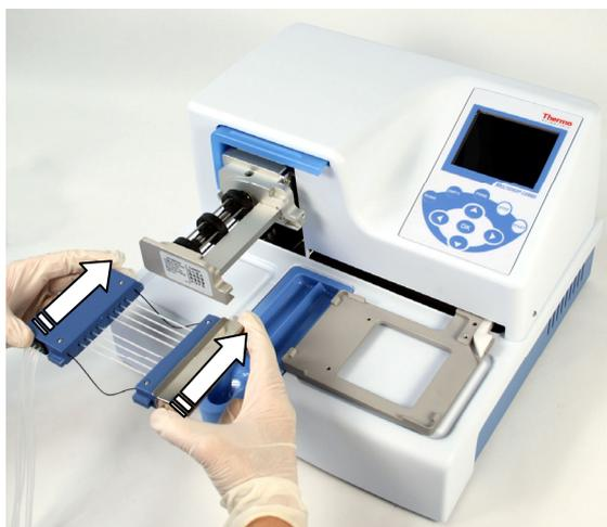
**Figure 4–11.** Inserting the dispensing cassette
