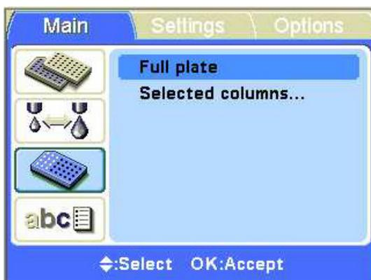
If you want to dispense into all the wells of the plate, select **Full plate** if it is not already shown on the screen. If you want to dispense only into some of the wells, select **Selected columns...** using the **Down** arrow key.
