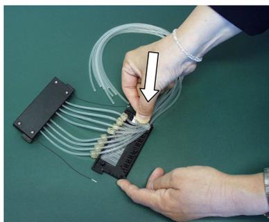
**Figure 5–36.** Pressing the tubing identification plate into place
