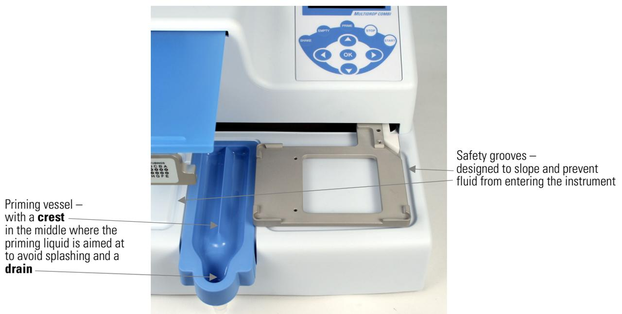
**Figure 4–9.** Priming vessel inserted into place
