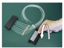
Figure 5–35. Placing the sight window
