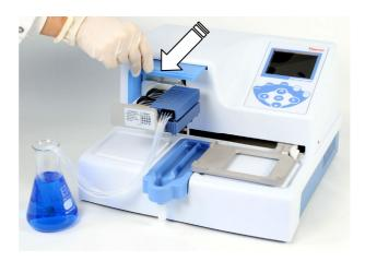
Figure 4–20. Pulling the rotor cover over the rotor
