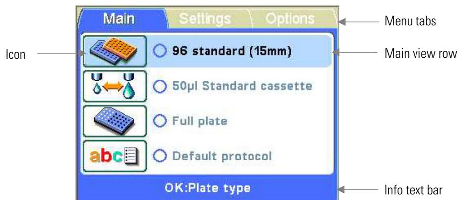
**Figure 4–22.** Main view on the display of the Multidrop Combi
