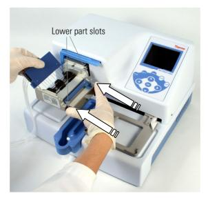
**Figure 4–12.** Inserting the lower part of the dispensing cassette into its slots
