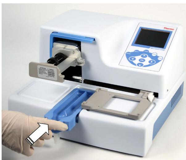
**Figure 3–8.** Inserting the priming vessel
