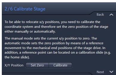
Figure 6. Step 2 of calibration
