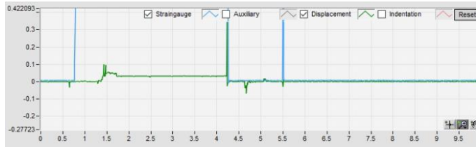
Figure 19: Find Surface options window. Piezo and cantilever signals during the “Find Surface” step.
