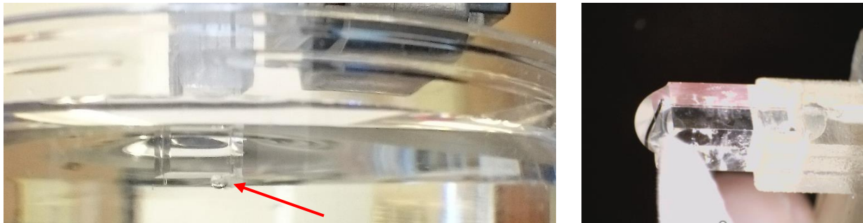
Figure 45: Side-view of an Optics11 probe while immersed in a transparent medium. As indicated by the red arrow, an air bubble is present at the base of the cantilever (left) and, Removing the air bubble by drying the probe (right).
