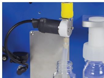
Figure 35. The drain tube on the condenser drain connector.
