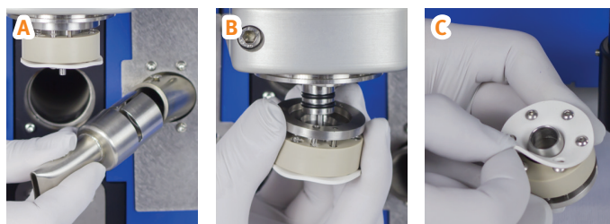
Figure 33. A: Removing the heater nozzle. B: Removing the upper vial holder. C: Loosening the vial face seal.
