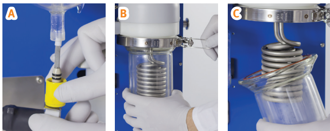
Figure 29. A: Removing the drain valve from the condenser pot. B: Loosening the clamp. C: Removing the condenser pot.
