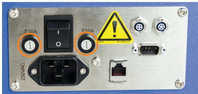
Figure 36. The fuse holders at the power inlet.
