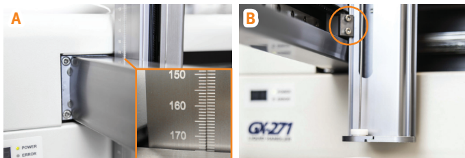
Figure 17. Ensure that the Z-arm is positioned at 175 mm (A). Adjust by loosening the two screws holding the arm in position (B).
