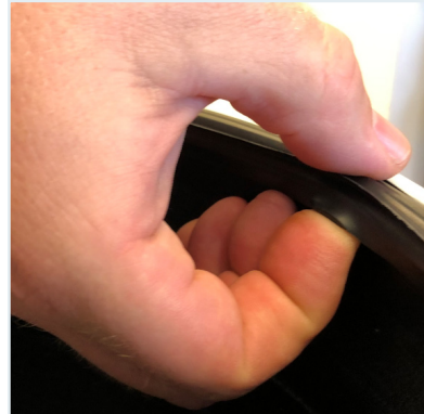
Hand position for seal removal
