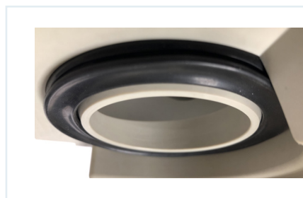
Condenser seal alignment with flange towards the bottom
