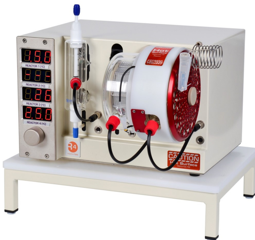
Figure 1 R4 Reactor Heater
