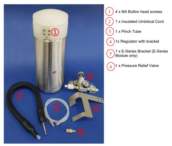
**Step 1** – Fit the regulator and bracket in the threaded holes using the 4 x M4 screws provided (See Fig 2). If being used with an E-Series module, the E-Series bracket also needs to be fitted (See Fig 3).
