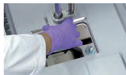
Hand guides Robotic Gripper Arm (RGA) to the correct centrifuge loading position below the deck using Zero-G technology.
