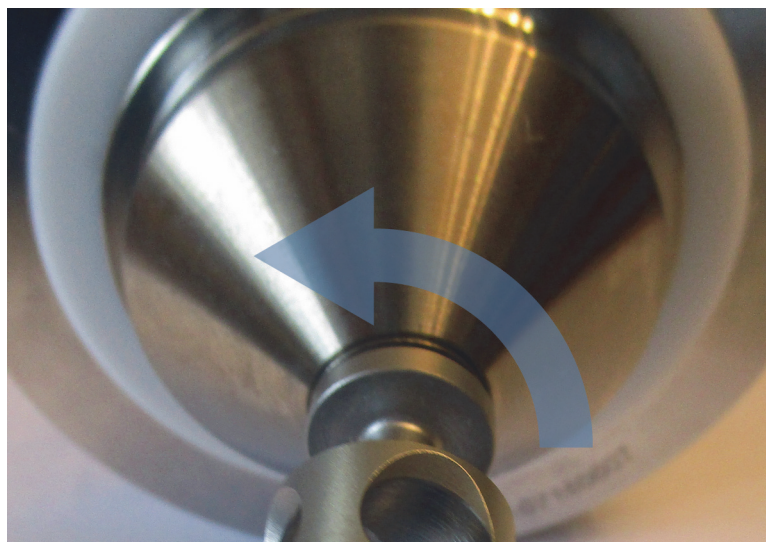
Figure 46. Turning the nose cone counterclockwise by a quarter turn (TSQ Altis MS)
