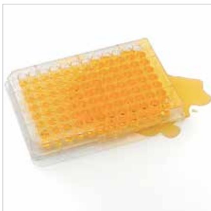
Spilling of plate caused by clogged needles
