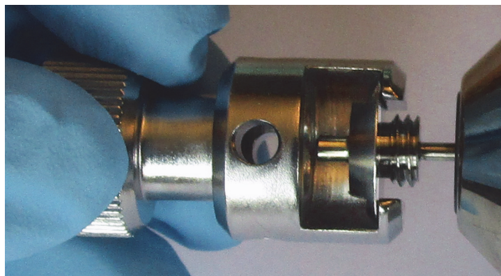
Figure 49. Pulling the tube out of the spray cone
