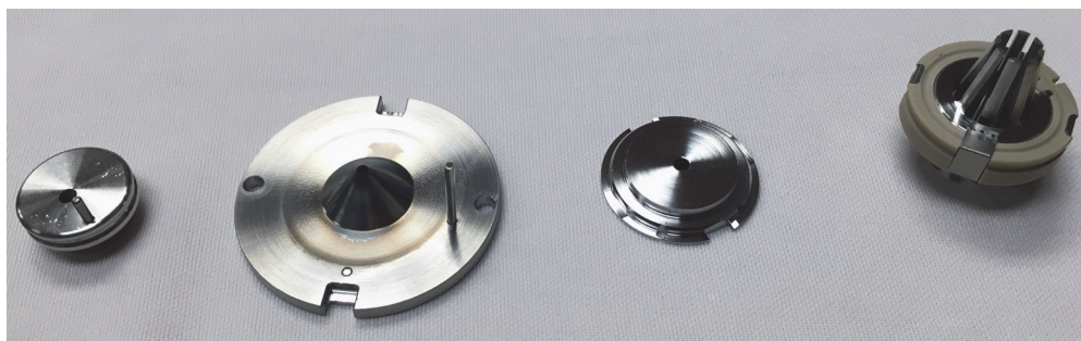
Figure 63. Tube lens, skimmer, L0 lens, and MP00 multipole (from left to right)
