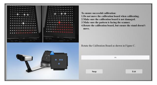
• The software will then prompt you to rotate the calibration board to match Orientation C. Carefully lift and rotate the calibration board without moving the stand.
