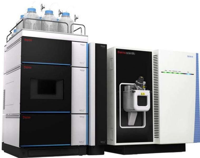
Thermo Fisher TSQ Altis inline triple quadrupole mass spectrometer coupled with an ultra-high-performance liquid chromatograph (UHPLC/MS/MS) for separation and analysis of synthesized bio-derived monomers. The device can accurately measure between 5-2000 m/z mass range with Active Ion Management. The device also contains 6 channel high-pressure solvent blending, allowing a variety of solvents to run through various columns depending on the compound.
