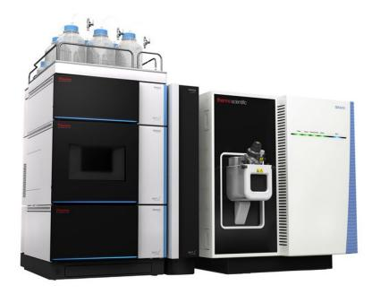
Thermo Fisher TSQ Altis inline triple quadrupole mass spectrometer coupled with an ultra-high-performance liquid chromatograph (UHPLC/MS/MS) for separation and analysis of synthesized bioderived monomers. The device can accurately measure between 5-2000 m/z mass range with Active lon Management. The device also contains 6 channel high-pressure solvent blending, allowing a variety of solvents to run through various columns depending on the compound.
