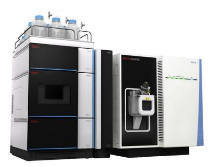
Thermo Fisher TSQ Altis inline triple quadrupole mass spectrometer coupled with an ultra-highperformance liquid chromatograph (UHPLC/MS/MS) for separation and analysis of synthesized bioderived monomers. The device can accurately measure betweeen 5-2000 m/z mass range with Active lon Management. The device also contains 6 channel high-pressure solvent blending, allowing a variety of solvents to run through various columns depending on the compound.
