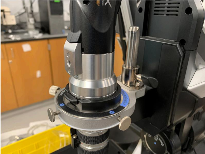
2. Twist the camera body counterclockwise and carefully lift directly off. Set carefully on its side to avoid damaging the lenses in the camera assembly
